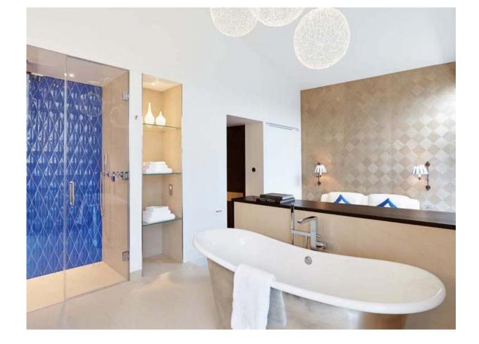
To combat regulation issues, there are three fiber-optic chandeliers above the bathtub that do not use electrics. They are lit from a projector housed outside of the room, so it means that there are no electrics above the bath tub. It's a safer alternative, and also created a mesmerizing effect when lit up - they can change color too for bathtub relaxation enjoyment.
